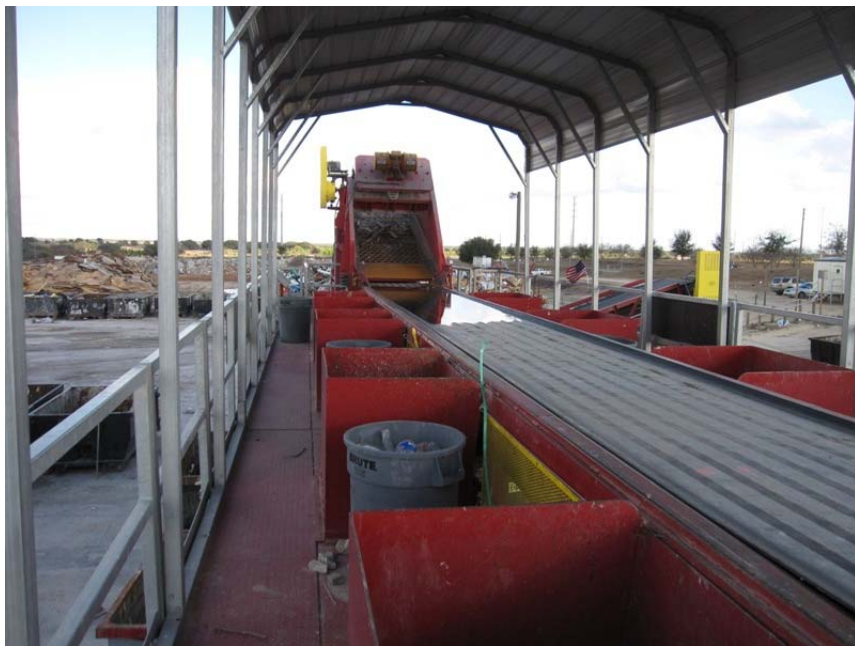
Picture 2 – MRF Conveyor and Sorting Stations
